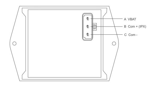
The Load Manager Voltage Input Module provides 4 inputs to the PMC system corresponding to specific battery voltages. In order to provide an accurate indication of system voltage, the Voltage Input Module should be located physically close to the vehicle's battery. *Care should be taken to minimize any voltage drop that may occur between the battery and the module.*
