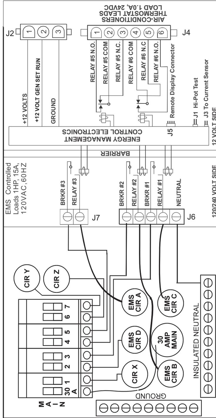
All 120VAC Shore Power must pass thru EMS Current Sensor.
