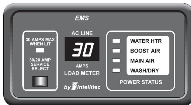
The optional display panel, can be mounted remotely and connects to the main unit with a small gauge, three wire cable.
