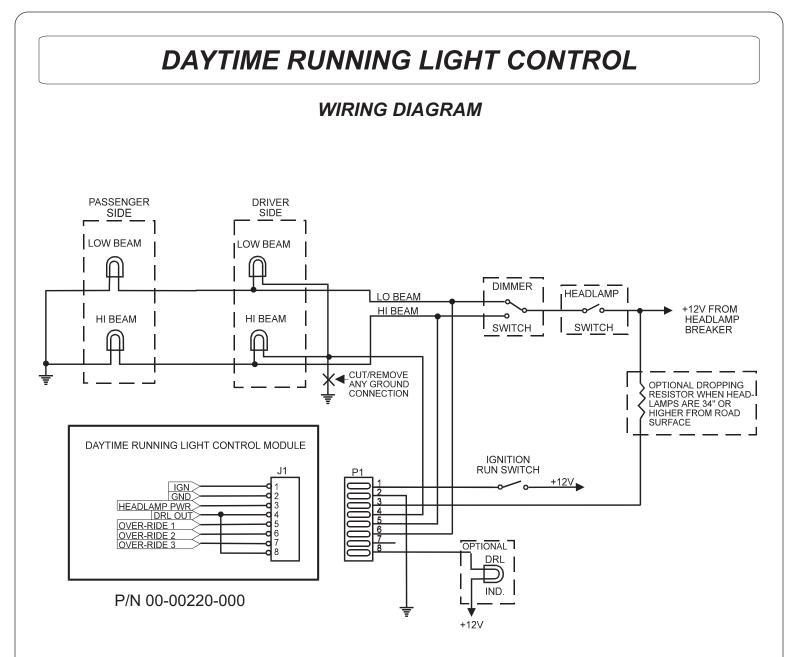
THE INTELLITEC DAYTIME RUNNING LIGHT CONTROL, AUTOMATICALLY WIRES THE HI BEAM HEADLAMPS IN SERIES AND TURNS THEM ON, APPROXIMATELY 20 SECONDS AFTER THE IGNITION SWITCH IS PLACED IN THE "RUN" POSITION. THE DRL INDICATOR WILL ILLUMINATE.
