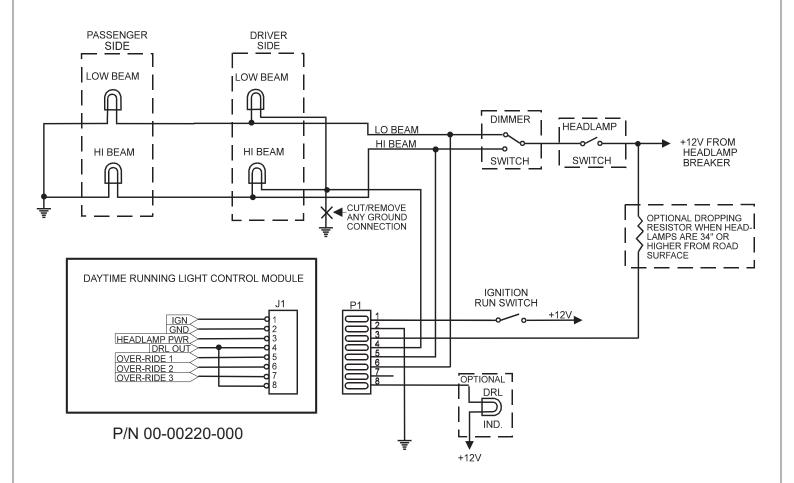
THE INTELLITEC DAYTIME RUNNING LIGHT CONTROL, AUTOMATICALLY WIRES THE HI BEAM HEADLAMPS IN SERIES AND TURNS THEM ON, APPROXIMATELY 20 SECONDS AFTER THE IGNITION SWITCH IS PLACED IN THE "RUN" POSITION. THE DRL INDICATOR WILL ILLUMINATE.
