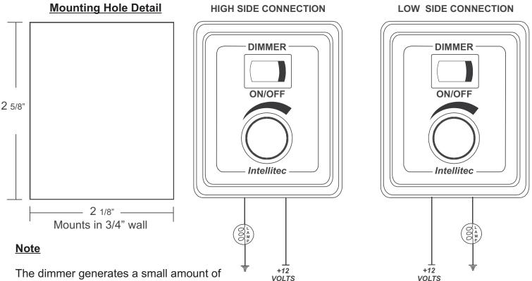
The dimmer generates a small amount of heat. To minimize temperature build-up when mounting the unit, be sure to provide at least 3 inches of space around the four sides of the unit for ventilation
