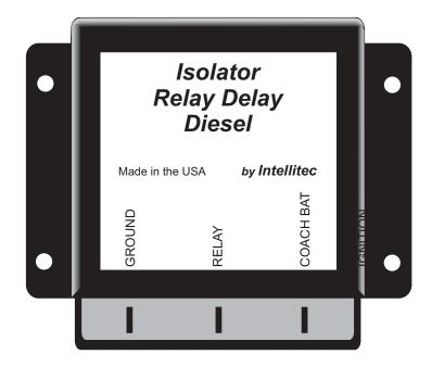
The unit is enclosed in a plastic housing for mounting in the engine compartment. It operates in combination with an intermittent duty cycle isolator relay, similar to ones used as diesel starter solenoids. There are three (3) wires to connect to the delay unit, one from an ignition switched 12 volt source, a ground and the isolator relay coil.
