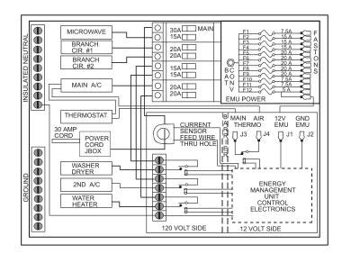
**EMU** senses the current drawn by all the loads in the RV and turns off selected loads if the total current exceeds a preset limit. It will hold the loads off until the total load current drops below a level that allows them to operate again.
