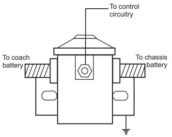
Note: This configuration is also common. The case is grounded to the body of the coach.
