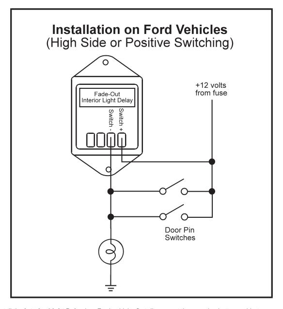
To Install the **Interior Light Delay** in a Ford vehicle, first disconnect the negative battery cable to prevent any damage to the wiring. Locate the two wires from any door pin switch (This can usually be done by removing the driver's or passenger's side kick panel.) and splice and tape a wire to each of these switch wires. *Do not cut the switch wire*. Crimp a 1/4" slip on connector to each of these wires and connect them to the Interior Light Delay module.
