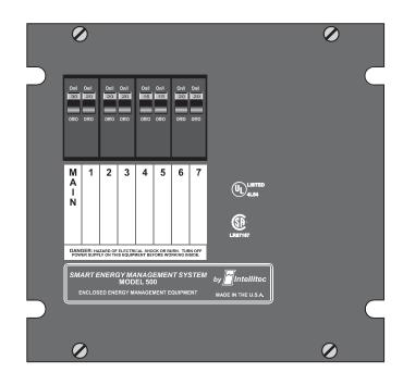
Smart EMS turns off each controlled appliance when the total current in the RV exceeds 30 amps. It will restore appliance power when the total current drops below a level that allows it to operate again.
