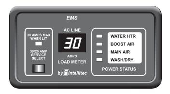
To help the owner understand what the system is doing, a series of LED's indicate the loads that have power applied. When the power is available, the LED will be on. There is a digital readout of the total amount of current being drawn by all the loads in the RV. The panel includes a switch to select operation from 30 amp or 20 amp service.
