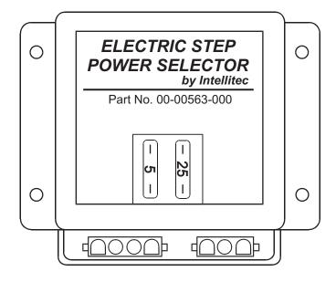
The Power Selector provides power to all three inputs (Step Power, Kill Switch, and Ignition) so that these levels are all compatible with the step control.
