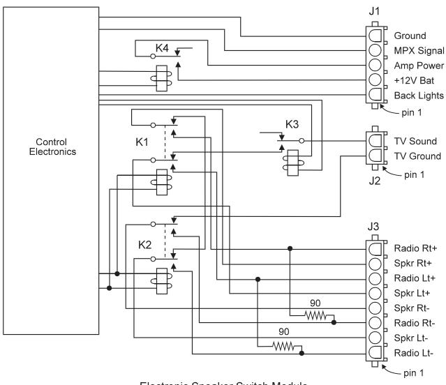
Electronic Speaker Switch Module Equivalent Circuit
