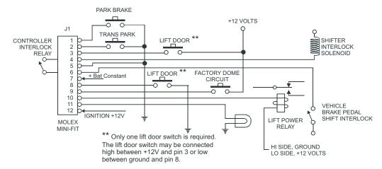
**Note:** The trans park input switch must be added to the vehicle so that the switch is in the closed position when the transmission is in park. For example, on a Ford E450, a switch bracket may be attached under the dash to interface with the shift indicator arm. (*Contact Intellitec for details*)
