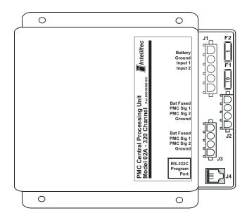
The CPU includes a sleep mode. The sleep mode reduces the overall system operating current, allowing the system to be constantly live with insignificant drain on the vehicle battery.
