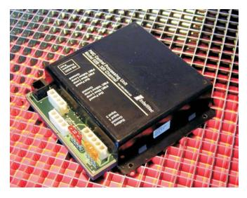
The CPU includes a sleep mode. The sleep mode reduces the overall system operating current, allowing the system to be constantly live with insignificant drain on the vehicle battery.
