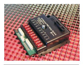
When using this module with PMC you should neither check the latched switch box in the Windows set up software for the pushbutton nor should a Boolean be written to operate the output. Channel P10 for 3 seconds will unlatch all latched outputs.
