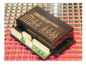
With the jumper closest to the edge of the board, the inputs will be high side. In other words, when the input is high, there will be an output on the PMC bus.
