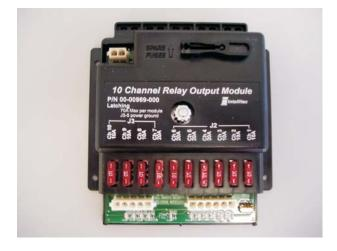
*written to operate the output.* Setting channel P10 for 3 seconds will unlatch all latched outputs.
