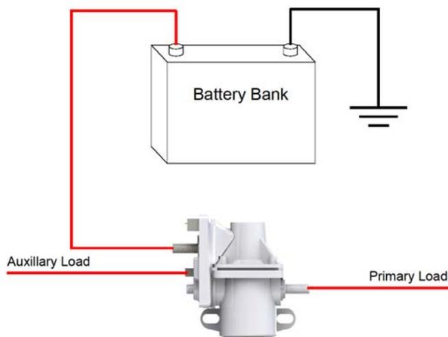
Wire Diagram 1 illustrates the primary connections of the Battery Guard® 1000. 5/16" bolts are used for the battery supply and Primary Load connections and are capable of supporting 100A of current. The Auxiliary Load uses a male ¼" quick connect and can supply up to 2A of current to the Auxiliary Load.
