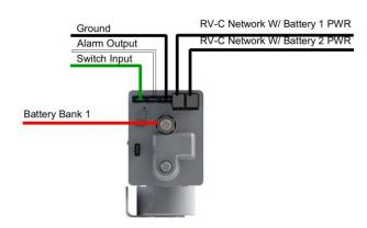
Wire Diagram 2 illustrates the additional connections on the B.I.R.D.®. Note that the second battery connection is on the opposite side of the device.
