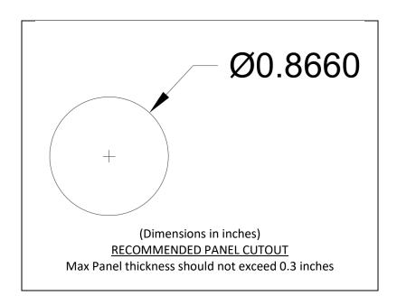
Note: Drawing dimensions refer to the switch used in the Intellitec kit (part # 10-01136-000).
