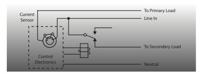
The AESS controls power to two loads. The primary or "on demand" load is connected to the primary output and a shed-able load is connected to the secondary output. The output to the secondary load is carried through a relay.
