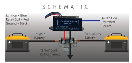
The Isolator Relay Delay operates in combination with a conventional continuous duty cycle isolator relay that has been used by a number of vehicle manufacturers. There are three (3) wires to connect to the delay unit: one from an ignition switched 12 volt source, a ground and the isolator relay coil.
