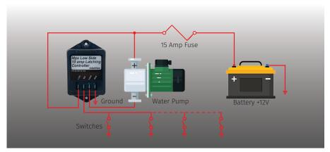
The Water Pump Controller is connected in the ground side of the water pump. The positive side of the pump is connected to a source +12 volts. The controller acts as the ground return for the pump.
