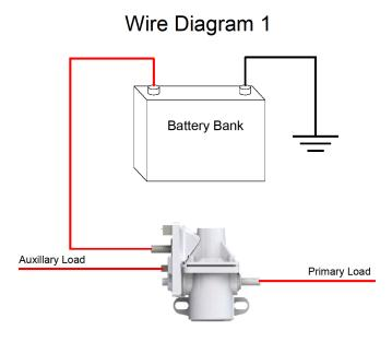
Wire Diagram 1 illustrates the primary connections of the Battery Guard® 1000. 5/16" bolts are used for the battery supply and Primary Load connections and are capable of supporting 100A of current. The Auxiliary Load uses a male \( \frac{4}{2} \) quick connect and can supply up to 2A of current to the Auxiliary Load.
