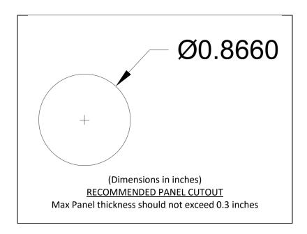
Note: Drawing dimensions refer to the switch used in the Intellitec kit (part # 10-01130-000).
