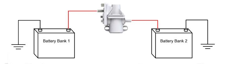
Wire Diagram 1 illustrates the primary connections of the B.I.R.D.®. 5/16" bolts are used for both battery supplies and are capable of supporting 100A of current.
