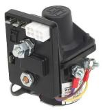
The B.I.R.D.® was designed to make installation simple. With its all in one integrated design, Intellitec brought the electronics to the source, eliminating additional wiring and simplifying the installation process. The B.I.R.D.® has a mounting plate attached with two mounting holes located in the back and uses automotive standard connectors for peripheral connections.
