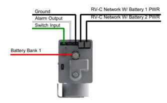
Wire Diagram 2 illustrates the additional connections on the B.I.R.D.®. Note that the second battery connection is on the opposite side of the device.
