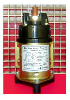
To close the Disconnect, a positive voltage is applied to the unmarked terminal of the coil and the negative of the supply is connected to the "S" terminal, for a brief period. When the power is removed, the relay is latched in the "on" or closed position. Current can now flow through the large terminals.
