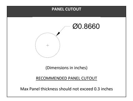
Note: If using switch as part of the Intellitec kit number 10-01153-000 refer to the dimensions above for mounting the switch in the wall.
