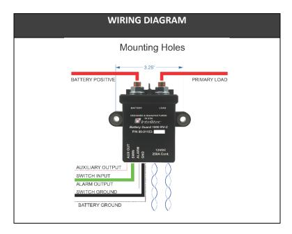
Note: Color combinations represented in the wiring diagram are from the 10-01153-000 kit harnesses. If using a different harness, please refer to the signal definitions when connecting to the device.
