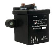
The HD Battery Guard® 1000 was designed to make installation simple. With its unique all in one design, Intellitec brought the electronics to the source, eliminating additional wiring and simplifying the installation process. The HD Battery Guard® 1000 has a mounting plate attached with two mounting holes located in the back and uses automotive standard connectors for peripheral connections.
